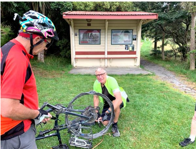
Neil and Tony repairing a tubeless tyre – notice how the tyre has collapsed and sucked inwards to itself by the internal “goop”
